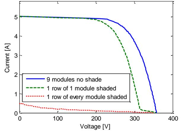
Fig. 2. I-V curves from string #1 (9 Sharp modules in series) when one row of cells in just one (out of 9) modules is shaded. The very low (red) curve corresponds to the case when the bottom row of each module in the string was shaded.
