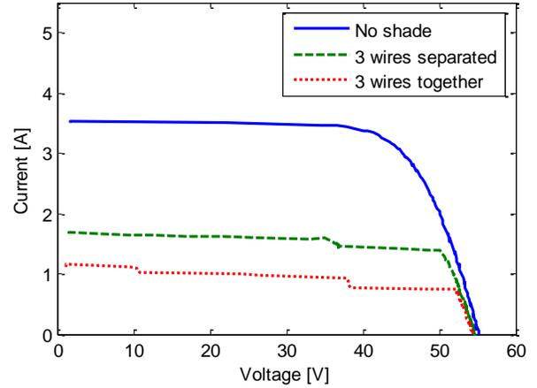
Fig. 5. I-V curves for one Sanyo module (from string #2) under the shade of three separated wires, three merged wires, and without shade.
