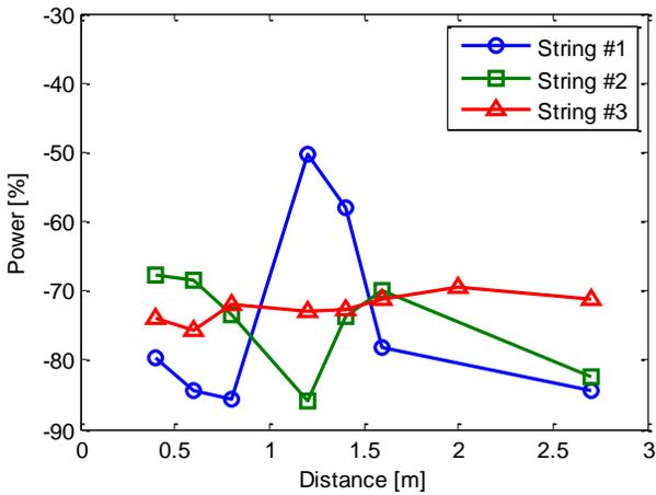
Fig. 7. Percent power loss  $[(P_{\text{shaded}} - P_{\text{normal}}) / P_{\text{normal}} * 100]$  vs. distance at which 4 wires are located from the surface of the module.
