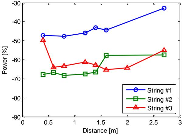
Fig. 6. Percent power loss  $[(P_{\text{shaded}} - P_{\text{normal}}) / P_{\text{normal}} * 100]$  vs. distance at which 2 wires are located from the surface of the module.
