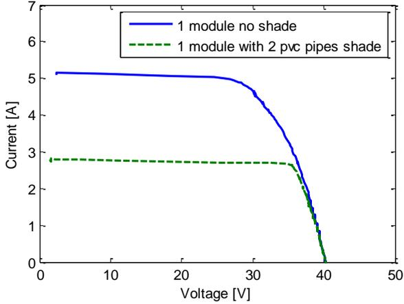
Fig. 4. I-V curves for a single Sharp module (from string #1) with shade from two bundled PVC pipes. When shaded by pipes the module's current is reduced.
