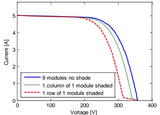
Fig. 3. I-V curves from string #1 with a column or a row shaded in just one (out of 9) modules.
